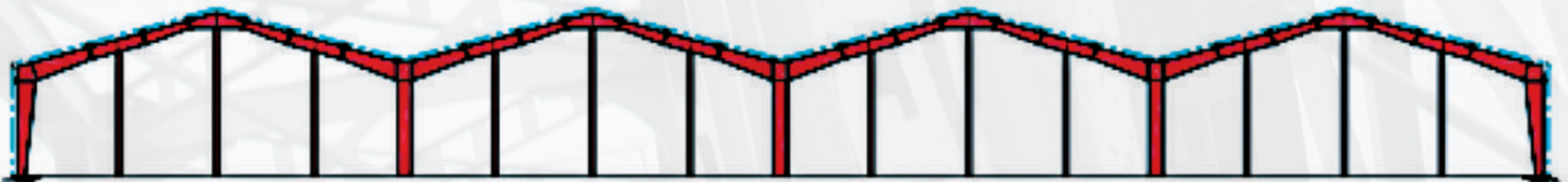
(CROSS SECTION) : MULTI-SPAN GABLE BLDG. WITH FOUR GABLES EACH W/ FOUR SPANS
