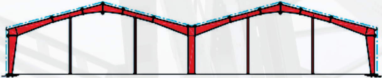
(CROSS SECTION) : MULTI-SPAN GABLE BLDG. WITH TWO GABLES EACH W/ THREE SPANS
