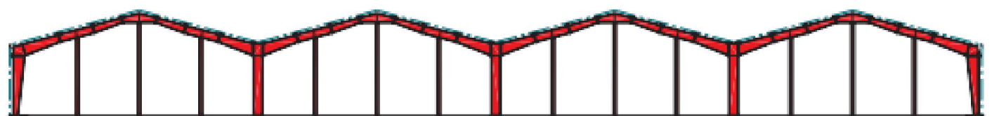
CROSS SECTION : MULTI-GABLE BLDG. WITH FOUR GABLES EACH W/ FOUR SPANS
